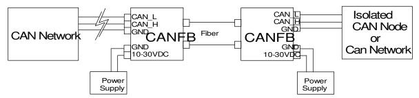
The CAN network must be terminated at both ends according to the CAN specification. Networks not properly terminated may have data errors or miss the data completely. The CANFBs create two new ends to the CAN network. Space is provided on the board for a termination resistor, R8. A 120-ohm resistor is recommended for the termination. If the CANFB is not at the end of the network, it should not be terminated.
