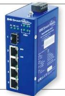
The **ESWP205-1SFP-T** is an industrial PoE+ Ethernet switch that complies with IEEE 802.3at standards. It provides four PoE+ 10/100Mbps copper ports supplying up to 30W of power to PD devices such as CCTV and WI-FI. An SFP port is available to support 100Mbps fiber SFPs.
