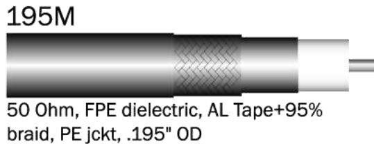
Figure 3-14 LMR195 Cable Cross Section
