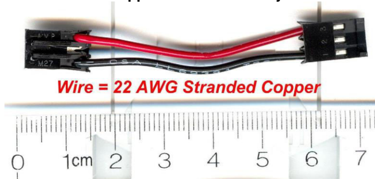
Figure 18. DC Wire Harness used to connect Striplight Boards. Note, this harness uses thicker gauge wire than would be used in a real, cost-sensitive commercial Striplight application, meaning that voltage drops seen in a real-world application would likely be worse than shown in Table 6.
