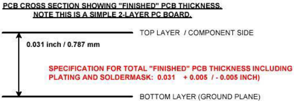
Figure 7. Cross-Section of +12 Volt Striplight PCB.
