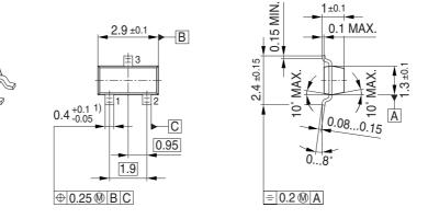
1) Lead width can be 0.6 max. in dambar area
