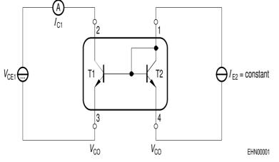
Note: Voltage drop at contacts:  $V_{CO} < 2/3 V_T = 16mV$
