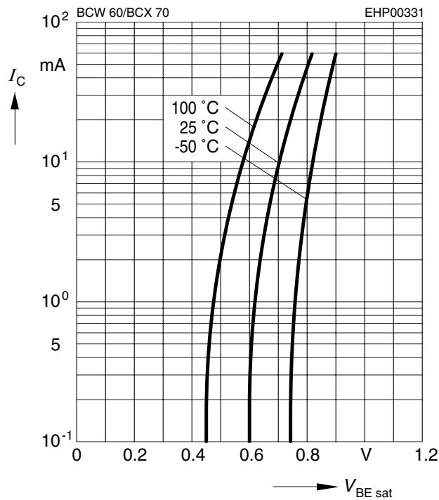
**Collector current**  $I_C = f(V_{BE})$
