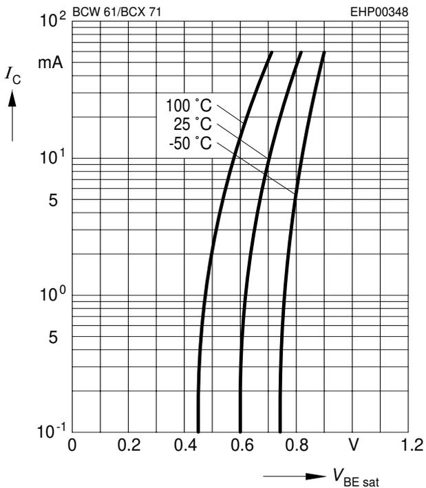
**Collector current  $I_C = f(V_{BE})$**
