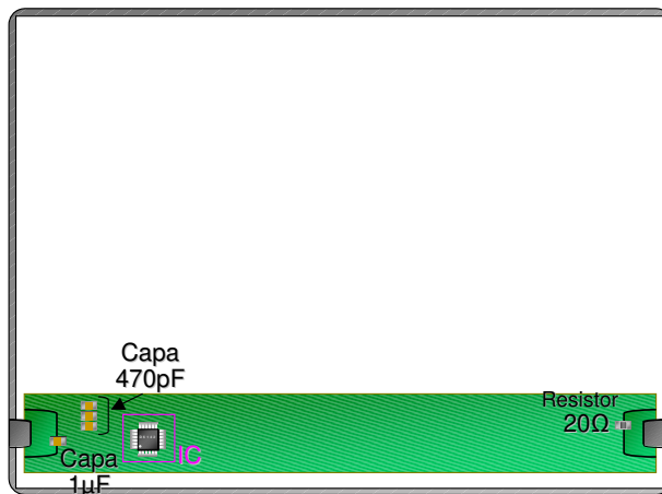
Figure 41. Layout example for ESD protection
