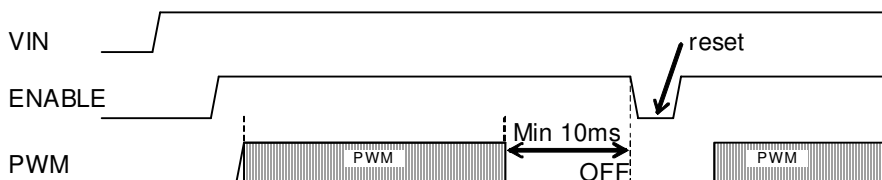
Figure 24. PWM stop and ENABLE turn “off”
