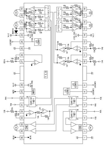
T.S.D: (Thermal shutdown) Resistance unit :  $[\Omega]$
