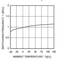
Fig. 8 Switching Frequency Temperature
