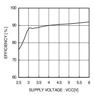
Fig. 18 Efficiency vs Power Supply Voltage
