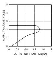
Fig. 14 VDD Load Regulation
