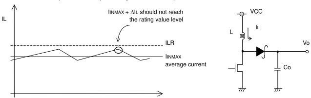
Fig. 27 Coil Current Waveform
