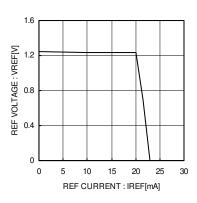
Fig. 5 Internal Reference Load Regulation
