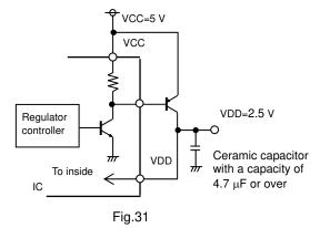
It is not necessary to use the regulator if the input voltage is 2.5 V. In that case, input 2.5 V to both VCC and VDD.
