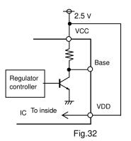
When incorporating a regulator into the external transistor, input the output voltage into the regulator.
