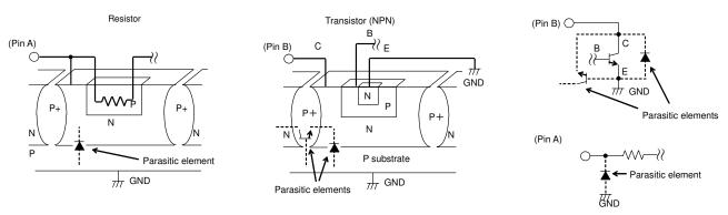
Fig.45 Example of a Simple Monolithic IC Architecture
