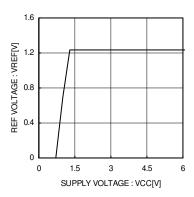
Fig. 4 Internal Reference Line Regulation
