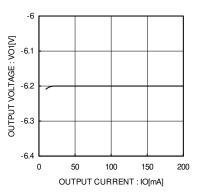
Fig. 23 Negative-side Charge Pump Load Regulation
