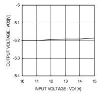
Fig. 22 Negative-side Charge Pump Line Regulation
