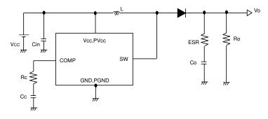
Fig. 30 Application Circuit Diagram
