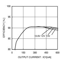
Fig. 17 Efficiency vs Output Current
