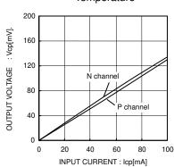
Fig. 11 Charge Pump On Voltage
