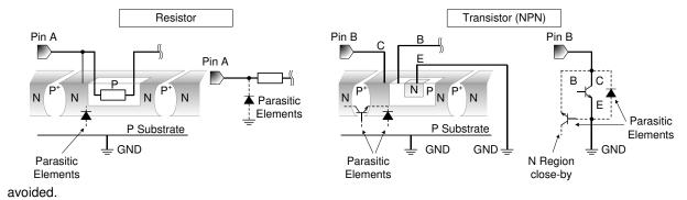
Figure 19. Example of monolithic IC structure
