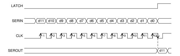
Figure 15. SEROUT Output Signal
