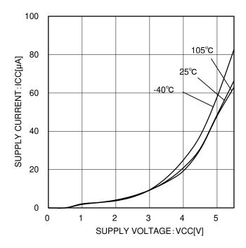
Figure 4. Circuit current (VCC characteristic)
