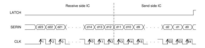
Figure 16. Cascade Connection
