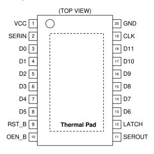
Figure 2. Pin Configuration
