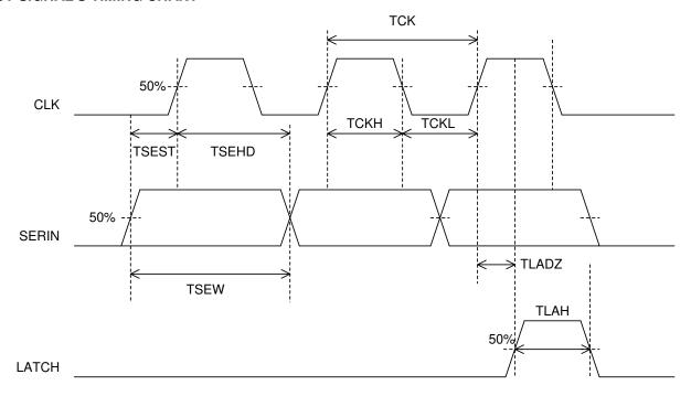
Figure 17. Timing Chart of Input Signal
