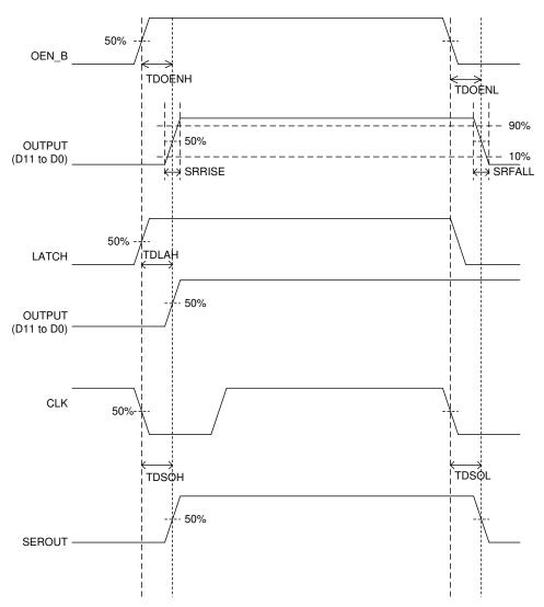
Figure 18. Delay Chart of Output Signal
