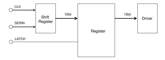
Figure 13. Block Diagram of Serial Communication
