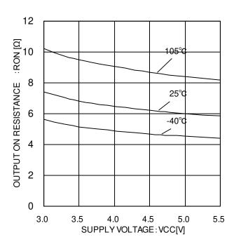
Figure 6. Output ON resistance (VCC characteristic @ ID=20mA)
