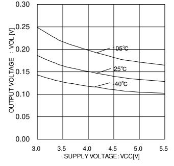
Figure 10. SEROUT high side voltage (Temperature characteristic @ ISO=-4mA)
