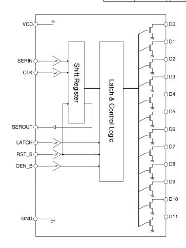
Figure 3. Block Diagram
