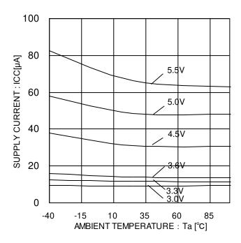
Figure 5. Circuit current (Temperature characteristic)
