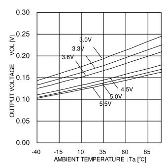
Figure 12. SEROUT low side voltage (Temperature characteristic @ ISO=4mA)
