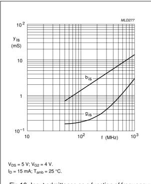
Fig.16 Input admittance as a function of frequency; typical values.
