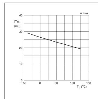
Fig.4 Transfer admittance as a function of the junction temperature; typical values.
