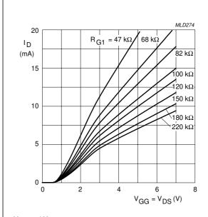
$V_{G2-S}$  = 4 V.  $R_{G1}$  connected to  $V_{GG}$ ;  $T_j$  = 25 °C.
