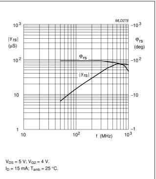
Fig.17 Reverse transfer admittance and phase as a function of frequency; typical values.
