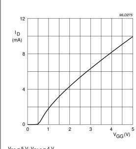
$V_{DS} = 5 \text{ V; } V_{G2\text{-}S} = 4 \text{ V.}$   $R_{G1} = 120 \text{ k}\Omega \text{ (connected to } V_{GG}); T_j = 25 \text{ °C.}$
