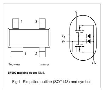
transistor consists of an amplifier MOS-FET with source and substrate interconnected and an internal bias circuit to ensure good cross-modulation performance during AGC.
