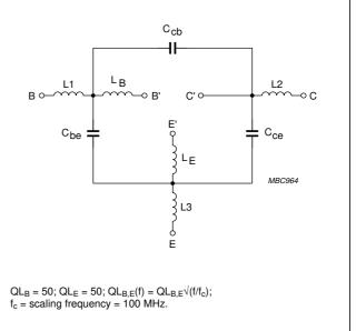
Fig.6 Package equivalent circuit SOT143.
