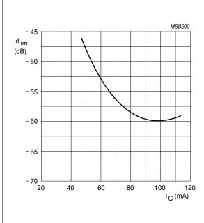
$$\begin{split} &V_{CE} = 10 \text{ V; } V_o = 900 \text{ mV; } T_{amb} = 25 \text{ °C;} \\ &f_{(p+q-r)} = 443.25 \text{ MHz.} \end{split}$$
