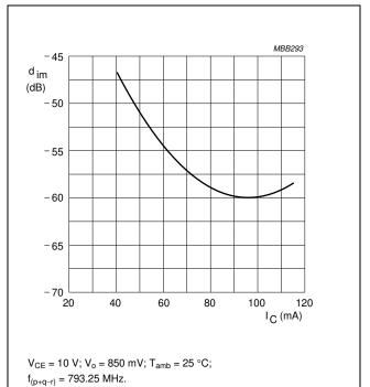
Fig.9 Intermodulation distortion as a function of collector current.
