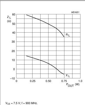
Fig.12 Load impedance as a function of output power.
