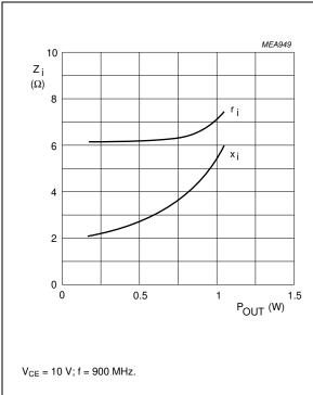
Fig.16 Input impedance as a function of output power.
