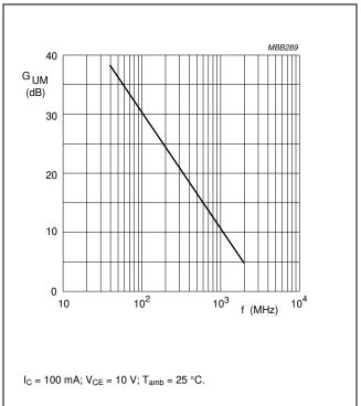
Fig.21 Maximum unilateral power gain as a function of frequency.
