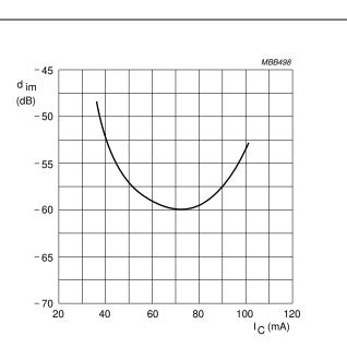
$$\label{eq:VCE} \begin{split} V_{CE} &= 8 \ V; \ V_o = 750 \ mV; \ T_{amb} = 25 \ ^\circ C; \\ f_{(p+q-r)} &= 443.25 \ MHz. \end{split}$$
