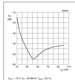
Fig.8 Second order intermodulation distortion as a function of collector current.
