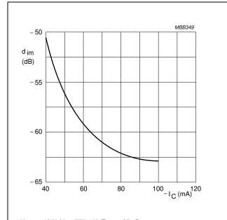
$V_{CE} = -10 \text{ V; } V_o = 550 \text{ mV; } T_{amb} = 25 \text{ °C; } \\ f_{(p+q-r)} = 848.25 \text{ MHz.}$
