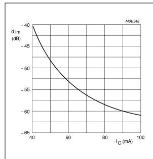
$V_{CE} = -10 \text{ V; } V_o = 650 \text{ mV; } T_{amb} = 25 \text{ °C; } \\ f_{(p+q-r)} = 443.25 \text{ MHz.}$
