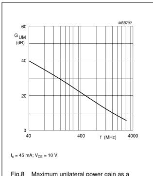
Fig.8 Maximum unilateral power gain as a function of frequency.
