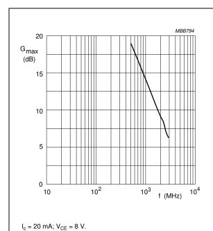
Fig.10 Maximum available stable gain as a function of frequency.
