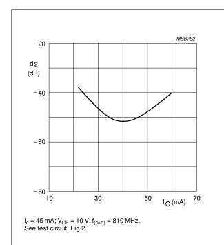
Fig.12 Second order intermodulation distortion as a function of collector current.
