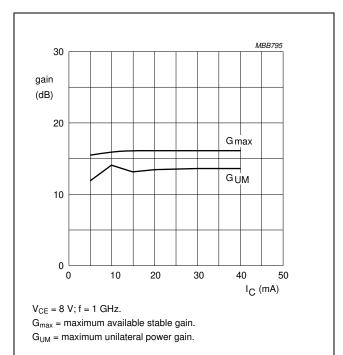
Fig.11 Gain as a function of collector current.
