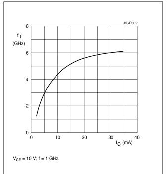
Fig.7 Transition frequency as a function of collector current.
