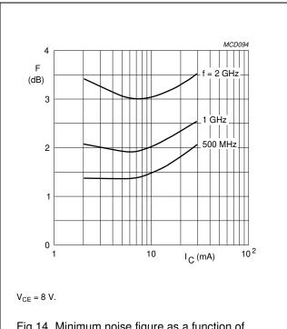
Fig.14 Minimum noise figure as a function of collector current.
