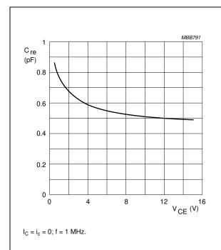
Fig.6 Feedback capacitance as a function of collector-emitter voltage.
