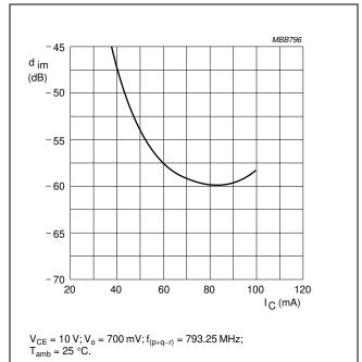
Fig.9 Intermodulation distortion as a function of
