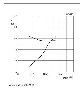
Fig.15 Input impedance as a function of output power.
