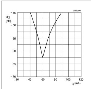
$V_{CE}$  = 10 V;  $V_{o}$  = 50 dBmV;  $f_{(p+q)}$  = 810 MHz;  $T_{amb}$  = 25 °C.
