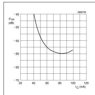
$\begin{aligned} &V_{CE} = 10 \text{ V; } V_o = 750 \text{ mV; } f_{(p+q-r)} = 443.25 \text{ MHz;} \\ &T_{amb} = 25 \text{ °C.} \end{aligned}$
