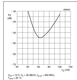
Fig.10 Second order intermodulation distortion as a function of collector current.
