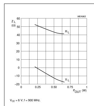
Fig.12 Load impedance as a function of output power.
