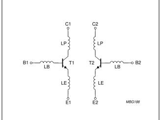
Fig.14 Package equivalent circuit SOT363A (inductance only).
