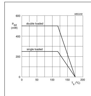
Fig.2 Power derating as a function of soldering point temperature; typical values.
