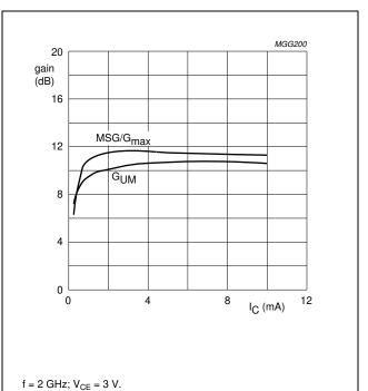
Fig.7 Gain as a function of collector current; typical values.
