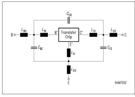
To avoid high complexity of the package equivalent circuit, both emitter leads of TSFP-4 are combined in one electrical connection. $R_{\rm LxI}$  are series resistors for the inductances  $L_{\rm xI}$  and  $K_{\rm xa-yb}$  are the coupling coefficients between the inductances  $L_{\rm xa}$  and  $L_{\rm yb}$ .
