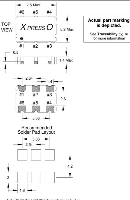
Note: XPRESSO LVDS VCXOs are designed to fit on Industry standard, 6 pad, layouts.
