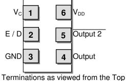
NOTE: XPRESSO LVDS VCXOs are designed to fit on Industry Standard, 6 pad layouts
