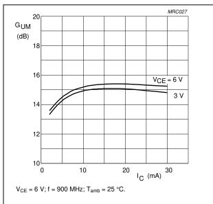
Fig.6 Maximum unilateral power gain as a function of collector current.
