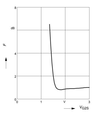
Noise figure  $F = f (V_{G2S})$ f = 800 MHz
