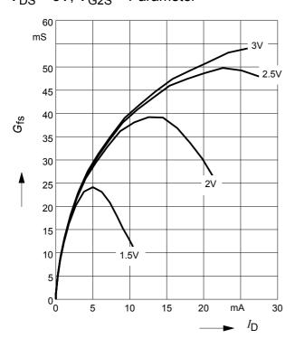
**Drain current**  $I_D = f(V_{GG})$  $V_{DS} = 3V$ ,  $V_{G2S} = 3V$ ,  $R_{G1} = 68k\Omega$ (connected to  $V_{GG}$ ,  $V_{GG}$ =gate1 supply voltage)
