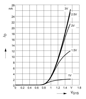
**Drain current**  $I_{\rm D} = f(V_{\rm GG})$
