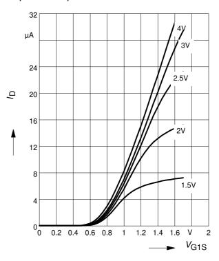
**Drain current**  $I_D = f(V_{GG})$  $V_{G2S} = 4V$ ,  $R_{G1} = Parameter in kΩ$ amp. A = amp. B
