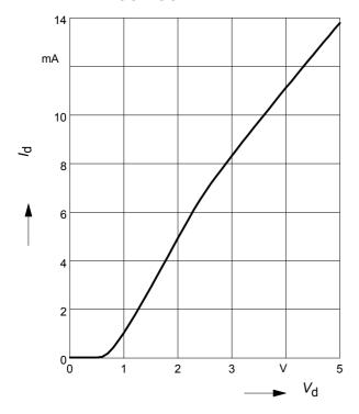
**Drain current**  $I_D = f(V_{G1S})$  $V_{DS} = 5V$ ,  $V_{G2S} = Parameter$
