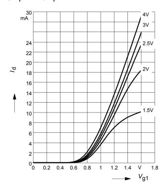
**Drain current**  $I_D = f(V_{GG})$
