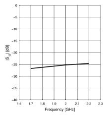
$$\begin{array}{lll} \textbf{Matching} & |S_{11}|, \ |S_{22}| = f(f) \\ V_{CC} = 2.78 V, \ I_{CC} = 6.5 mA \end{array}$$
