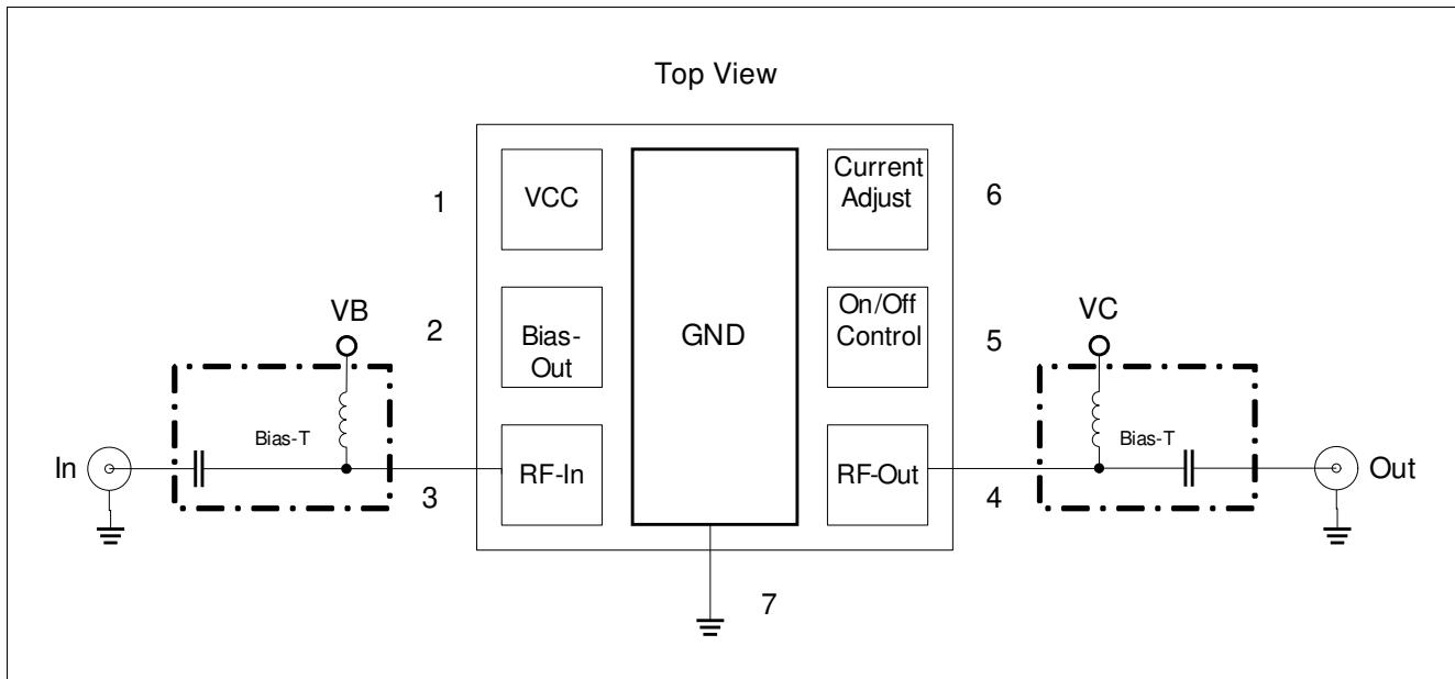
**Figure 8-5 Testing Setup**
