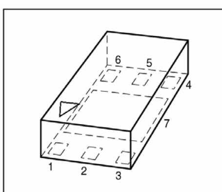
Figure 3-1 Pin Configuration
