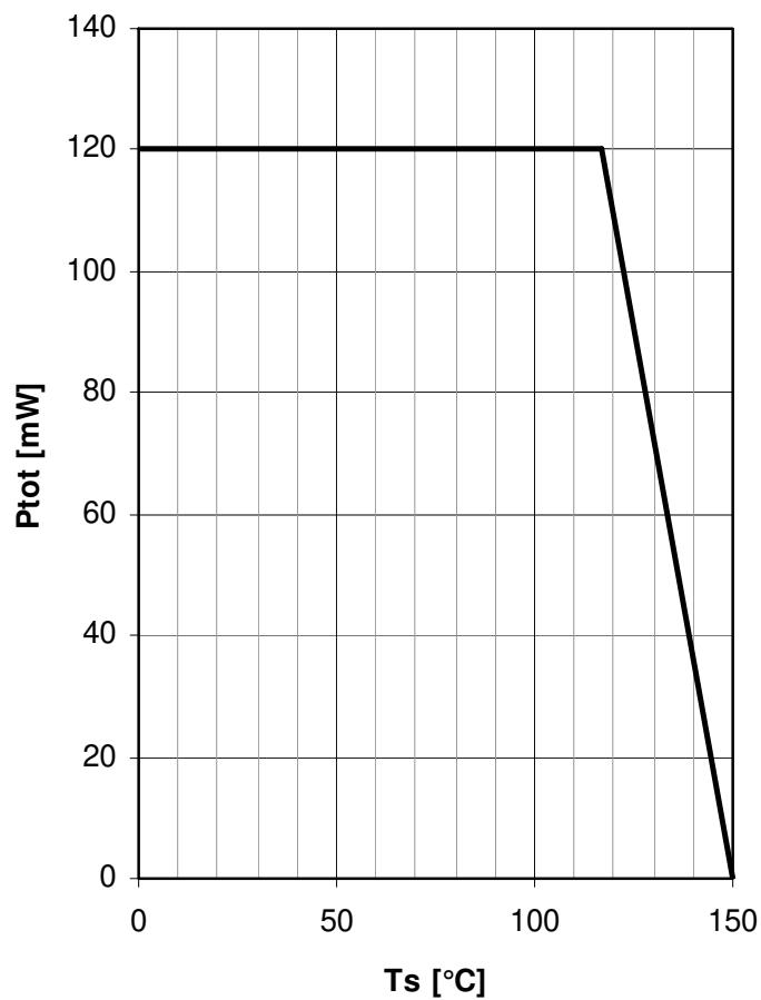
**Figure 7-1 Maximum Total Power Dissipation  $P_{tot}$  as Function of Temperature  $T_s$  at Soldering point**
