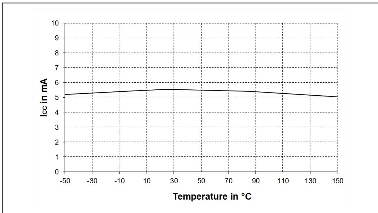
**Figure 8-4**  $I_{CC}$  as a Function of Temperature,  $V_{CC} = 3$  V,  $V_{Ctrl} = 3$  V,  $R_{ext} = \text{open}$
