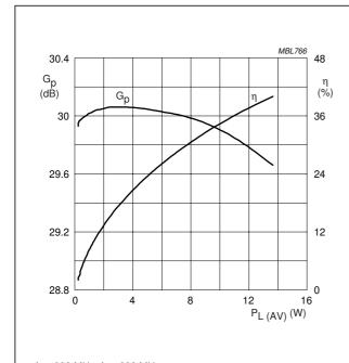
$f_1 = 882 \text{ MHz}; f_2 = 883 \text{ MHz}.$
