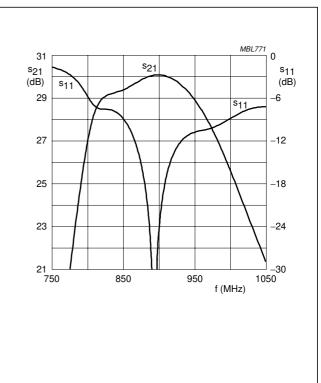
Fig.11 s-parameters as a function of frequency.
