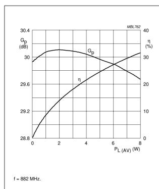
Fig.2 IS95 power gain and efficiency as functions of load power; typical values.
