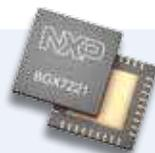
The BGX7221 combines a pair of high-performance, high-linearity down-mixers for use in receivers that have a common local oscillator used with, for example, main and diversity paths. The device covers frequency bands from 1700 to 2700 MHz with an extremely flat behavior.
