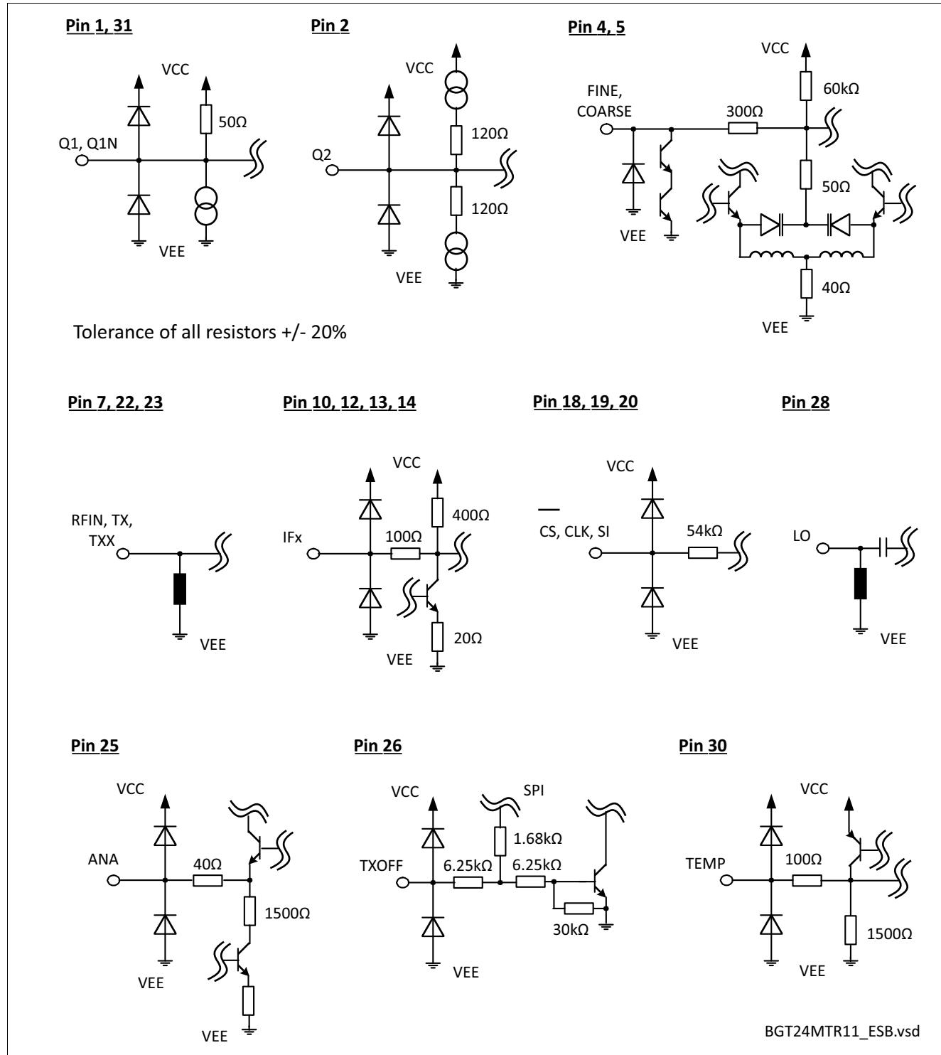
Figure 7 Equivalent Circuit Diagram of MMIC Interfaces
