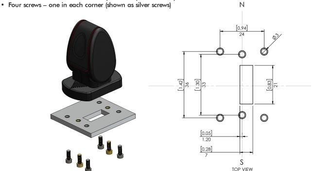
The Paddle is fitted with M3 bushes in all six positions, as standard. Fasteners are not supplied as standard. The appropriate length of fastener is dependent on panel thickness.
