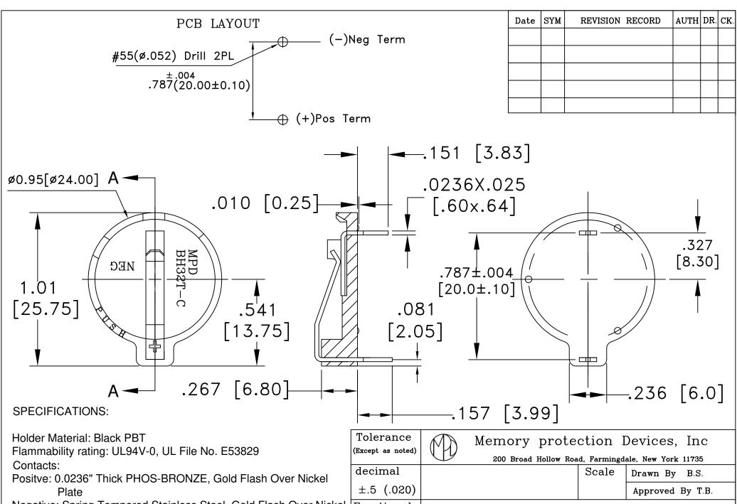
Negative: Spring Tempered Stainless Steel, Gold Flash Over Nickel Temperature Range: -40°C to +140°C **ROHS COMPLIANT**
