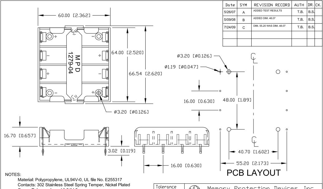
Cover: Polypropylene, UL94V-0 Heat Deflection Temperature: 90°C
