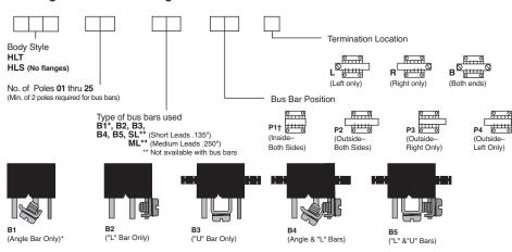
Angle Bar mounts on common or center terminals only. mum of 4 Poles Required.
