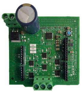
system solution footprint. An SPI interface is provided for parameter setting and monitoring the system health and utilized through the PCA9655E's 16 bits of General Purpose parallel Input and Output (GPIO) expansion.
