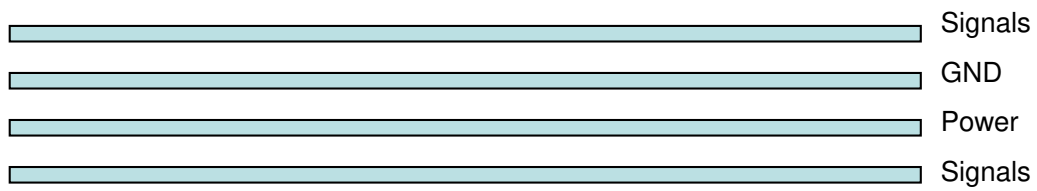
Figure 15: Typical 4-layer PCB construction
