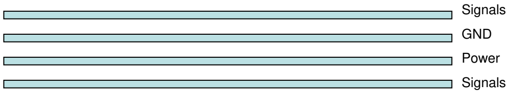
Figure 12: Typical 4-layer PCB construction
