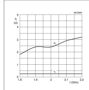
$V_{DS}$  = 26 V;  $I_{DQ}$  = 180 mA;  $P_L$  = 45 W;  $T_h \leq$  25 °C.
