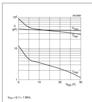
Fig.2 Input, output and feedback capacitance as functions of drain-source voltage, typical values.
