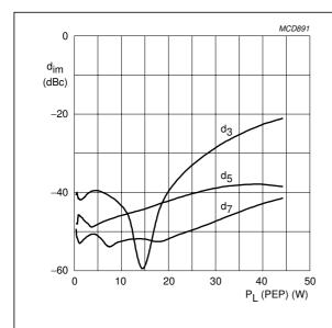
$$\begin{split} V_{DS} = 26 \text{ V; } I_{DQ} = 180 \text{ mA; } T_h \leq 25 \text{ °C;} \\ f_1 = 2000 \text{ MHz; } f_2 = 2000.1 \text{ MHz.} \end{split}$$
