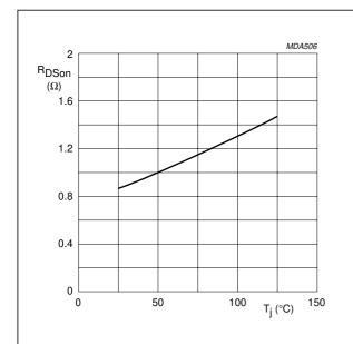
$I_D = 1.2 A$ ;  $V_{GS} = 10 V$ .
