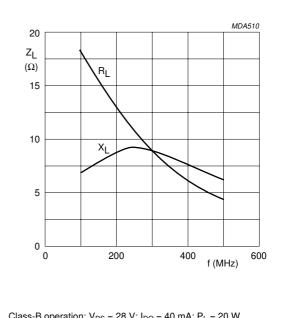
Class-B operation;  $V_{DS}$  = 28 V;  $I_{DQ}$  = 40 mA;  $P_L$  = 20 W.
