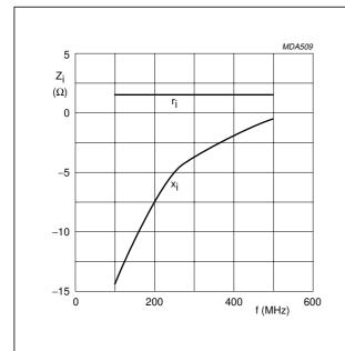
Class-B operation;  $V_{DS}$  = 28 V;  $I_{DQ}$  = 40 mA;  $P_{L}$  = 20 W.
