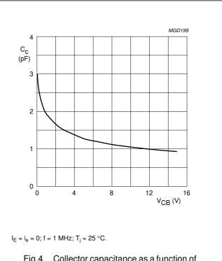
Fig.4 Collector capacitance as a function of collector-base voltage; typical values.
