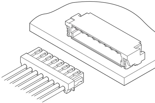
**The world's first 0.8mm pitch wire-to-board insulation displacement connector. Side entry type is only 3.9mm depth and 1.75mm height after mounting on the PC board, and top entry type is only 2.2mm depth and 3.9mm height. Compared to the conventional 1.0mm pitch SSR connector, occupation space on the board is reduced by 34% (side entry type).**
