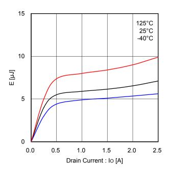
Figure 25. Low Side Recovery Loss (VDC=300V)
