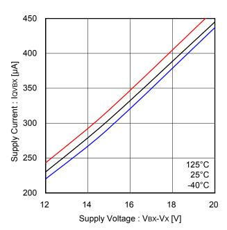
Figure 17. High Side Driver Operating Current (F<sub>PWM</sub>: 20kHz, Each Phase)
