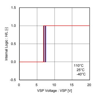
Figure 31. Testing Mode Threshold Voltage
