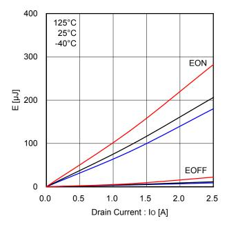
Figure 24. Low Side Switching Loss (VDC=300V)
