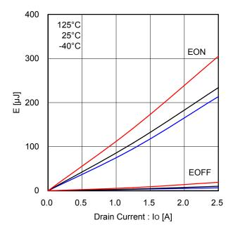
Figure 22. High Side Switching Loss (VDC=300V)
