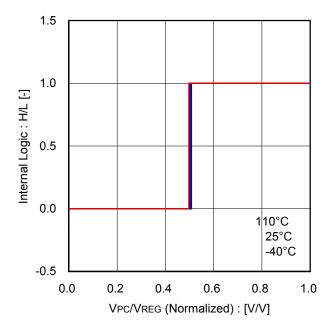
Figure 34. PWM Switching Arm Threshold Voltage
