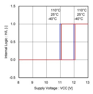
Figure 45. Under Voltage Lock Out (Low Side Drivers)
