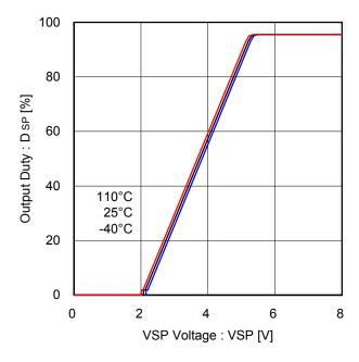
Figure 30. Output Duty - VSP Voltage (PC=H)
