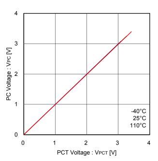
Figure 33. PCT - PC Linearity (RPCT=RPC= $100k\Omega$ )
