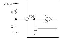
Figure 9. Release Time Setting Application Circuit
