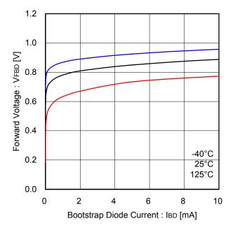
Figure 20. Bootstrap Diode Forward Voltage
