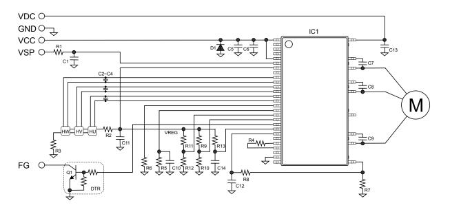
Figure 46. Application Example (120° Commutation Driver)
