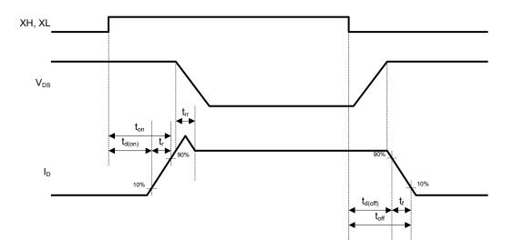
Figure 11. Switching Time Definition
