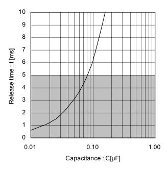
Figure 10. Release Time (Reference Data @R=100kΩ)
