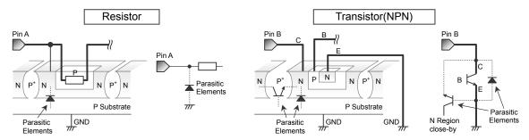
Figure A-1. Example of IC structure
