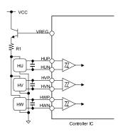
Figure 5. VREG Output Pin Application Example
