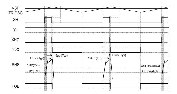
Figure 8. Fault Operation ~ OCP ~ Timing Chart
