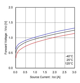
Figure 19. Output MOSFET Body Diode
