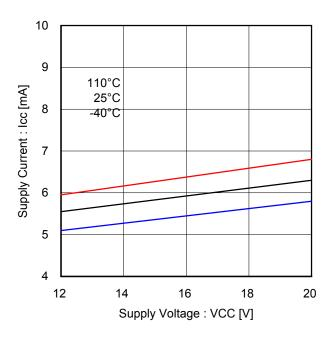
Figure 15. Low Side Drivers Operating Current (F<sub>PWM</sub>: 20kHz)
