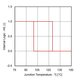
Figure 43. Thermal Shutdown
