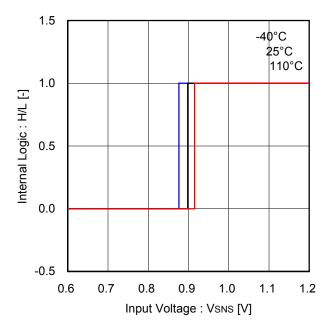
Figure 42. OCP Input Threshold Voltage (SNS)
