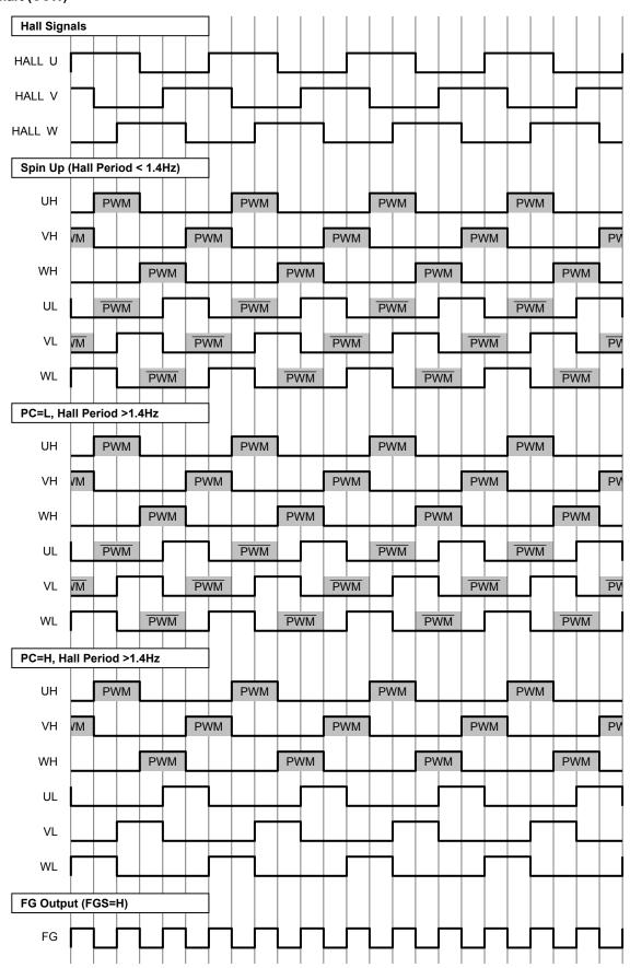
Figure 13. Timing Chart (Counter Clockwise)
