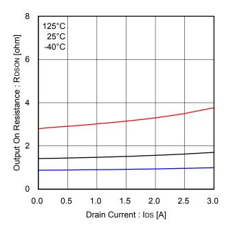
Figure 18. Output MOSFET ON Resistance
