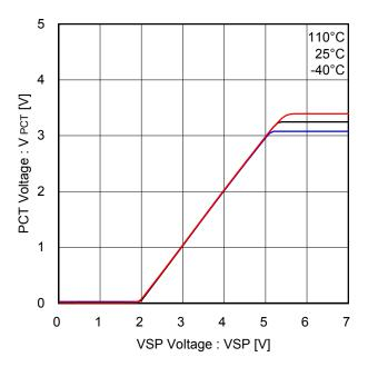
Figure 32. VSP - PCT Offset Voltage
