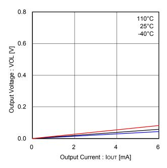
Figure 37. Low Side Output Voltage (FG)
