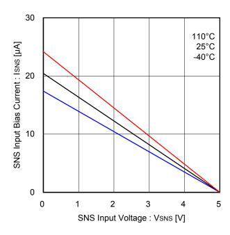
Figure 40. SNS Input Bias Current
