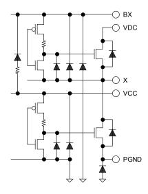
Figure 57. VCC, PGND, VDC, BX(BU/BV/BW), X(U/V/W)
