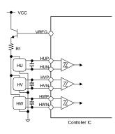
Figure 6. VREG Output Pin Application Example
