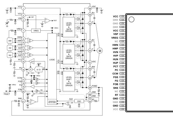
Figure 2. Block Diagram
