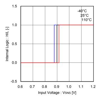
Figure 43. OCP Input Threshold Voltage (SNS)
