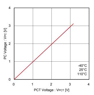
Figure 34. PCT - PC Linearity (RPCT=RPC= $100k\Omega$ )
