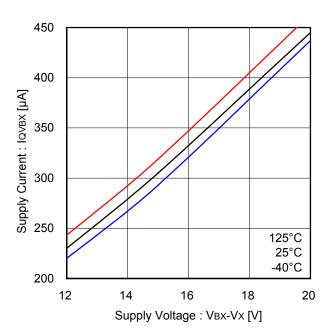
Figure 18. High Side Driver Operating Current (F<sub>PWM</sub>: 20kHz, Each Phase)
