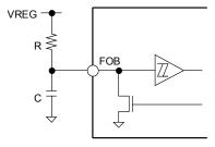
Figure 10. Release Time Setting Application Circuit
