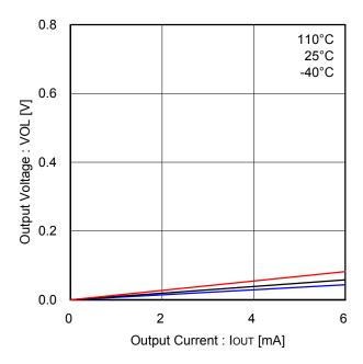
Figure 38. Low Side Output Voltage (FG)
