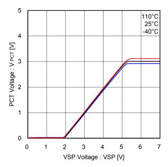
Figure 33. VSP - PCT Offset Voltage
