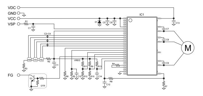
Figure 47. Application Example (180° Sinusoidal Commutation Driver)
