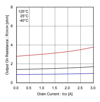
Figure 19. Output MOSFET ON Resistance
