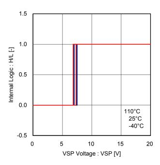
Figure 32. Testing Mode Threshold Voltage
