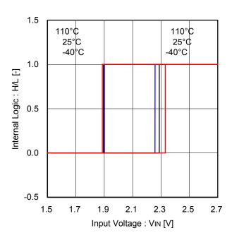
Figure 40. Input Threshold Voltage (CCW, FGS, FOB)
