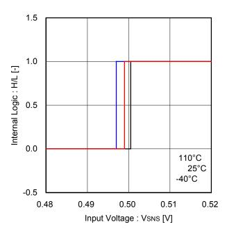
Figure 42. Current Limiter Input Threshold Voltage (SNS)
