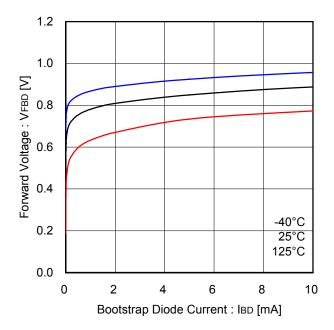
Figure 21. Bootstrap Diode Forward Voltage
