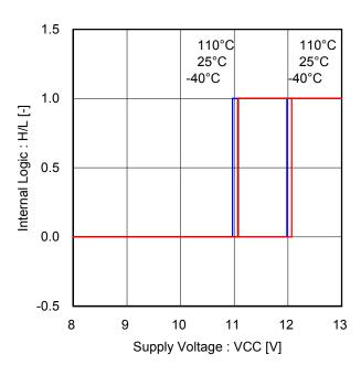
Figure 46. Under Voltage Lock Out (Low Side Drivers)
