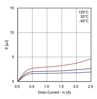
Figure 24. High Side Recovery Loss (VDC=300V)
