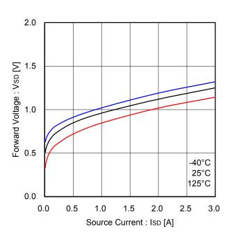
Figure 20. Output MOSFET Body Diode
