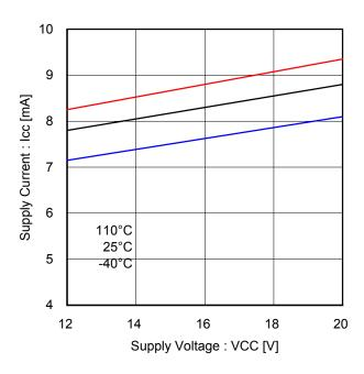
Figure 16. Low Side Drivers Operating Current (F<sub>PWM</sub>: 20kHz)
