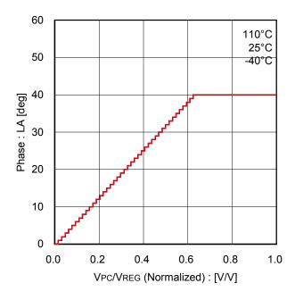
Figure 35. PC Voltage Normalized - Lead Angle
