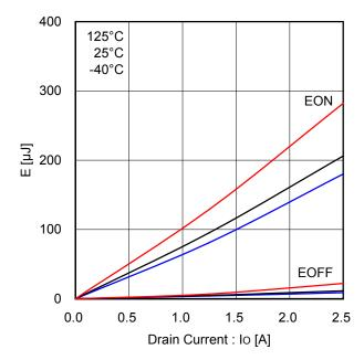
Figure 25. Low Side Switching Loss (VDC=300V)
