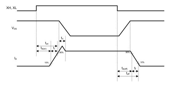
Figure 12. Switching Time Definition
