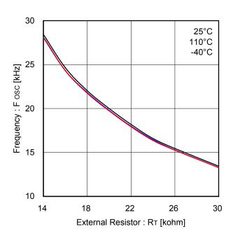
Figure 36. Carrier Frequency - RT
