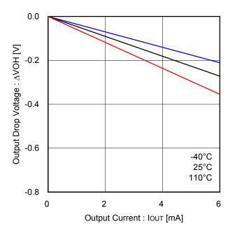
Figure 37. High Side Output Voltage (FG)
