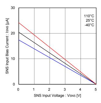
Figure 41. SNS Input Bias Current
