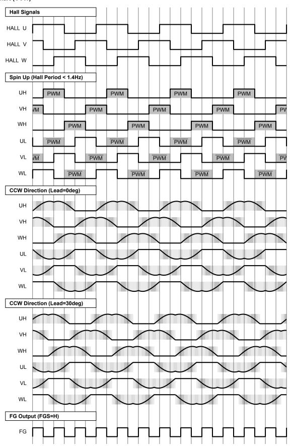
Figure 14. Timing Chart (Counter Clockwise)
