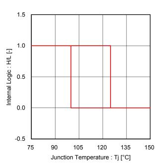
Figure 44. Thermal Shutdown
