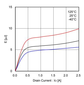
Figure 26. Low Side Recovery Loss (VDC=300V)
