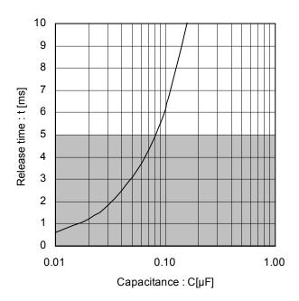
Figure 11. Release Time (Reference Data @R=100kΩ)
