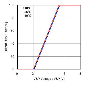
Figure 31. Output Duty - VSP Voltage
