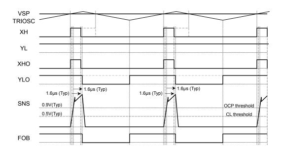
Figure 9. Fault Operation ~ OCP ~ Timing Chart
