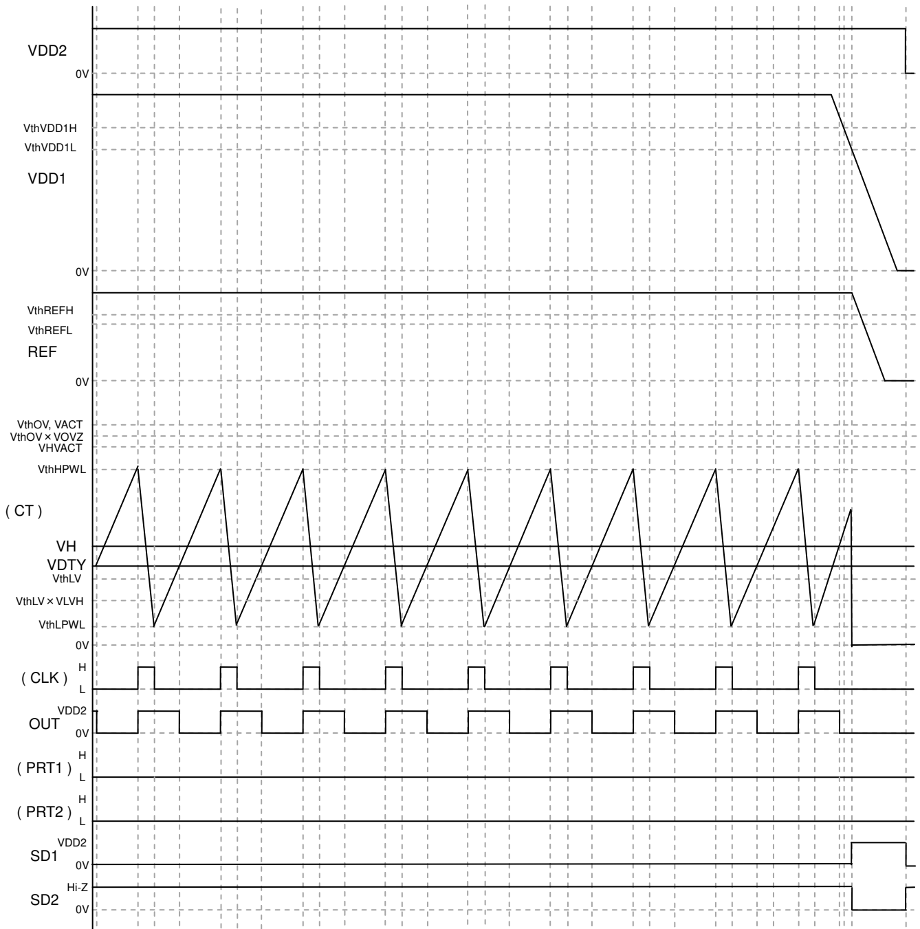
Figure 5. VDD1 Stop to VDD2 Stop Timing Chart
