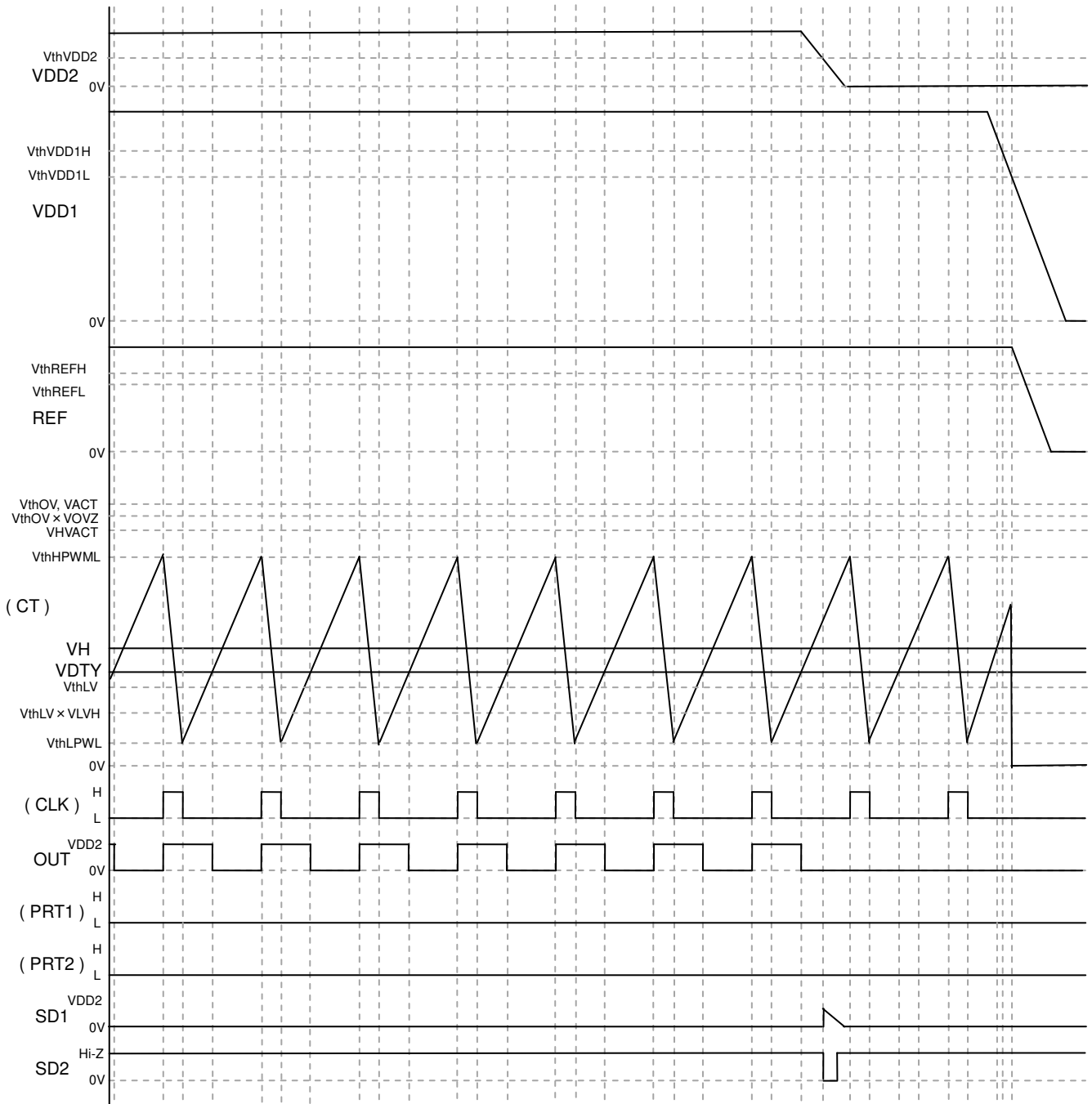
Figure 6. VDD2 Stop to VDD1 Stop Timing Chart
