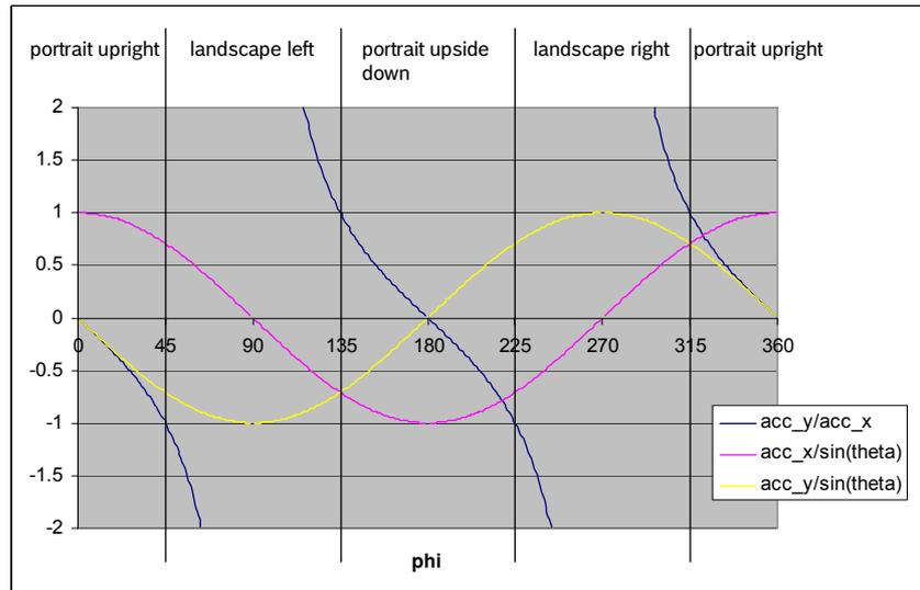
The criteria for portrait/landscape switching is fulfilled and the interrupt is generated when the threshold  $|acc\_y/acc\_x|=1$  is crossed (i.e.  $45^\circ$ ,  $135^\circ$ ,  $225^\circ$ ,  $315^\circ$ ). As soon as the interrupt is set, no new interrupt is generated within the hysteresis level of  $0.66 < |acc\_y/acc\_x| < 1.66$  corresponding to a hysteresis interval of  $\pm 13\%$  around the threshold.
