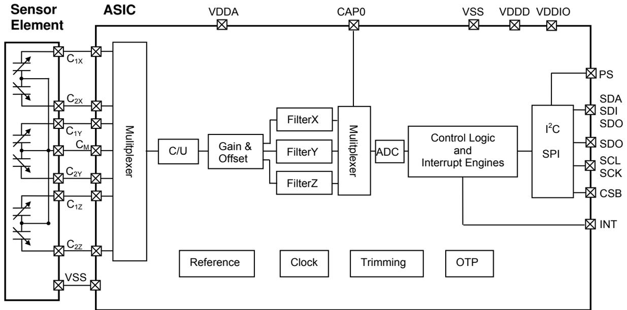
Figure 1: Block diagram BMA220
