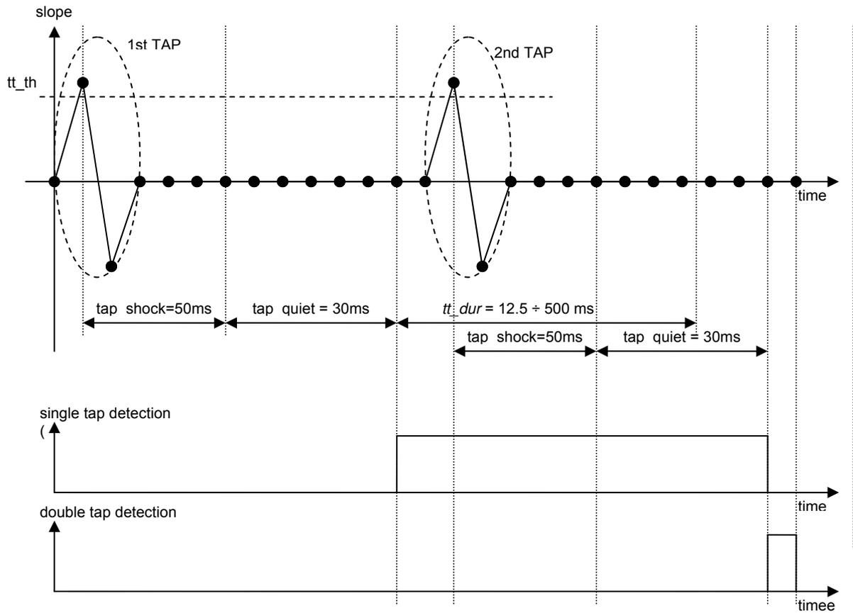
When a tap-sensing interrupt is triggered, the following details can be read from the corresponding registers: the axis that has triggered the interrupt ( $tt\_first\_x$ ,  $tt\_first\_y$ ,  $tt\_first\_z$ ) and the motion direction of the triggering acceleration signal ( $tt\_sign$ ).
