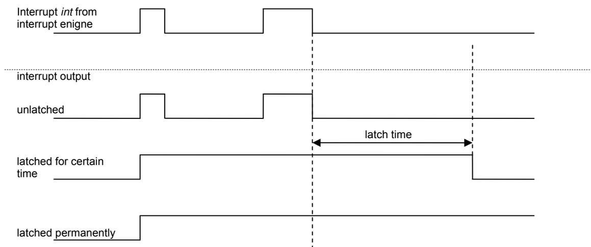
Figure 5: Interrupt output
