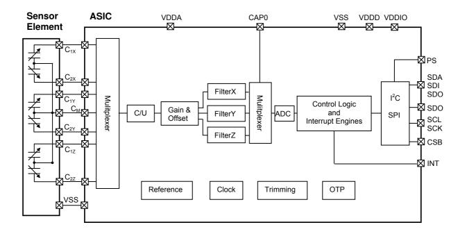
Figure 1: Block diagram BMA220
