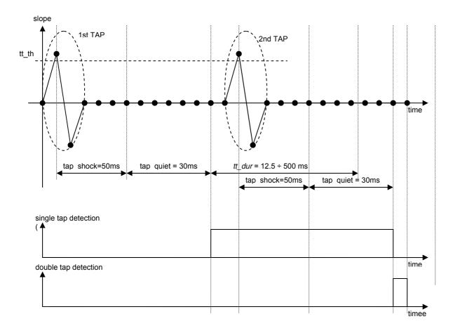
When a tap-sensing interrupt is triggered, the following details can be read from the corresponding registers: the axis that has triggered the interrupt ( $tt_first_x, tt_first_y, tt_first_z$ ) and the motion direction of the triggering acceleration signal ( $tt_sign$ ).
