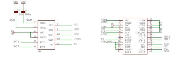
BMA222E shuttle board electrical layout
