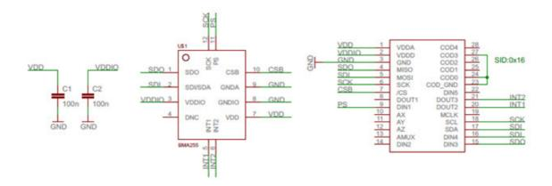
BMA280 shuttle board electrical layout
